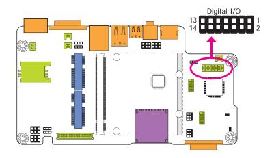
The 12-bit Digital I/O connector provides powering-on function to external devices that are connected to the connector. The pin functions of the digital I/O connector are listed below:
