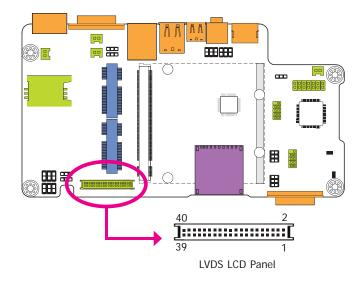
The system board allows you to connect a LCD Display Panel by means of the LVDS LCD panel connector transmitting video signals and power from the system board to the LCD Display Panel.
