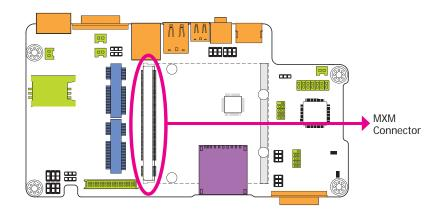
The MXM connector is used to interface the carrier board with a Oseven board. Refer to the table in the following pages for the pin functions of the MXM connector.
