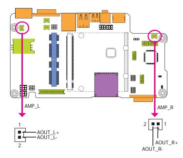
The amplify right/left connectors which have amplifying feature are used to connect external speakers.
