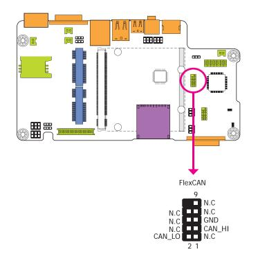
The CAN controller performs communication in accordance with the BOSCH CAN Protocol Version 2.0B Active1 (standard format and extended format). The bit rate can be programmed to a maximum of 1Mbit/s. To connect the CAN controller module to the FlexCAN connector, it is necessary to add transceiver hardware.
