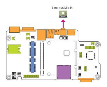
The system board is equipped with 1 audio jack to operate as a line-out jack or a mic-in jack. A jack is a one-hole connecting interface for inserting a plug. Being a line-out jack, this jack is used to connect a headphone or external speakers. Being a mic-in jack, this jack is used to connect to the center and subwoofer speakers of the audio system.
