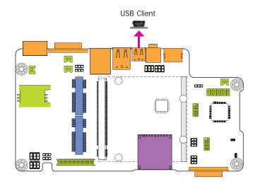
The shape of the mini USB port is smaller than the standard one and is a device operating as a client port.
