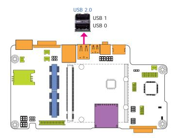
The USB device allows data exchange between your computer and a wide range of simultaneously accessible external Plug and Play peripherals. The system board is equipped with two onboard USB 2.0 ports (USB 0-1).
