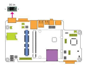
This jack provides maximum of 60W power and is considered a low power solution. Connect a DC power cord to this jack. Use a power adapter within 12~36V DC output voltage. Using a voltage out of the range 12~36V may fail to boot the system or cause damage to the system board.
