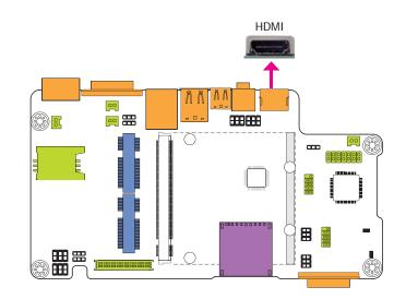
The HDMI port which carries both digital audio and video signals is used to connect a LCD monitor or digital TV that has the HDMI port.
