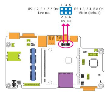
JP7 and JP8 allow you to select the audio function. When pins 1-2, 3-4, and 5-6 are set to On, JP7 is applied for the Line-out function and JP8 is used for the Mic-in function.
