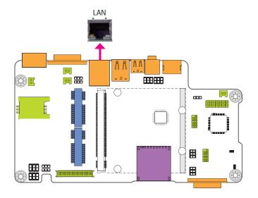
The onboard RJ45 LAN port allows the system board to connect to a local area network by means of a network hub.
