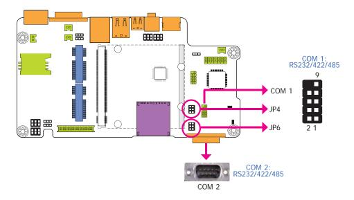
JP4 (for COM 1) and JP6 (for COM 2) are used to configure the COM ports to RS232, RS422 (Full Duplex) or RS485. The pin functions of COM ports will vary according to jumpers' setting.
