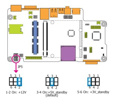
JP5 is used to select the power level of the LCD/inverter power connector.
