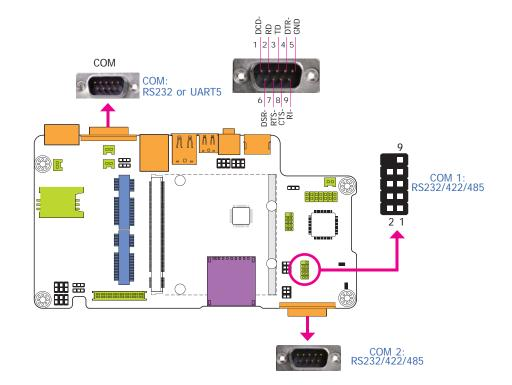
The system board is equipped with two onboard serial COM ports (COM and COM 2). It is also equipped with a 9-pin connector for connecting an external serial COM port (COM 1). COM is fixed at RS232 or UART5 via JP11's and JP12's setting at the same time. COM port 1 and COM port 2 will vary according to JP4's (for COM 1) and JP6's (for COM 2) setting respectively.
