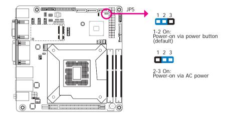
JP5 is used to select the method of powering on the system. If you want the system to power on whenever AC power comes in, set JP5 pins 2 and 3 to On. If you want to use the power button, set pins 1 and 2 to On.
