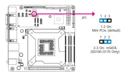
JP1 is used to select the Mini PCIe signal.
