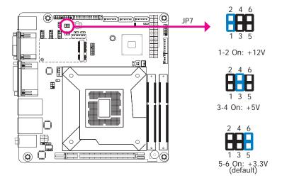
JP7 is used to select the power supplied with the LCD panel.
