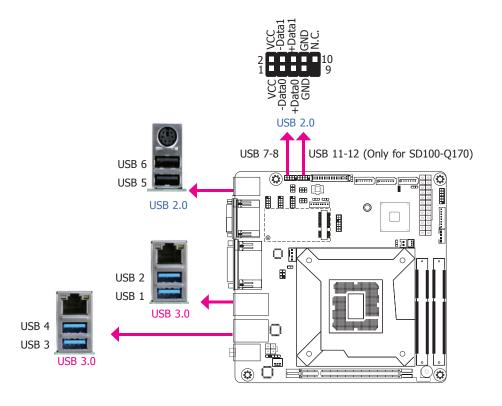
The USB device allows data exchange between your computer and a wide range of simultaneously accessible external Plug and Play peripherals.
