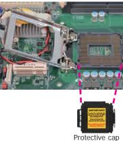
7. Insert the CPU into the socket. The gold triangular mark on the CPU must align with the corner of the CPU socket shown on the photo.
