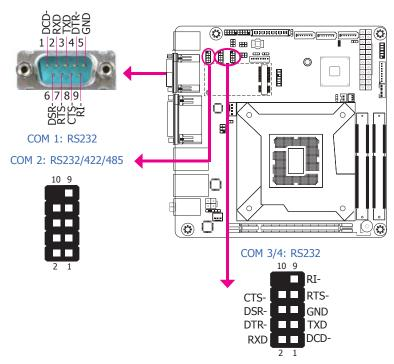
COM 1, COM 3 and COM 4 are fixed at RS232. COM 2 can be selected among RS232, RS422 and RS485 via the BIOS setup utility.
