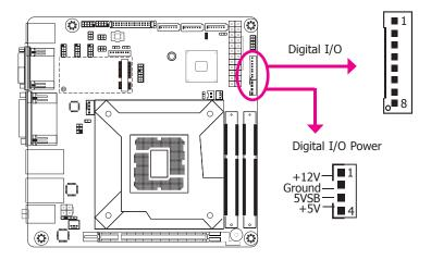
The 8-bit Digital I/O connector provides powering-on function to external devices that are connected to these connectors.
