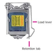
Lifting the load lever will at the same time lift the load plate.
