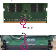
6. Grasping the module by its edges, position the module above the socket with the "notch" in the module aligned with the "key" on the socket. The keying mechanism ensures the module can be plugged into the socket in only one way.
