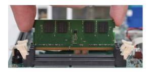
7. Seat the module vertically, pressing it down firmly until it is completely seated in the socket. The ejector tabs at the ends of the socket will automatically snap into the locked position to hold the module in place.
