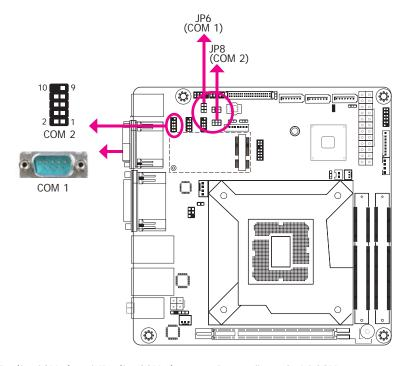
JP6 (for COM 1) and JP8 (for COM 2) are used to configure Serial COM ports to pure RS232 or RS232 with power. The pin functions of COM 1 and COM 2 will vary according to JP6's and JP8's setting respectively.
