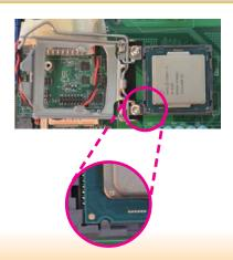
8. Close the load plate then push the load lever down.
