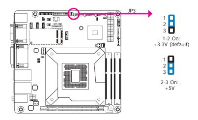
JP3 is used to select the power level of backlight brightness control: +3.3V (default) or +5V.
