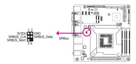
The SMBus (System Management Bus) connector is used to connect SMBus devices. It is a multiple device bus that allows multiple chips to connect to the same bus and enable each one to act as a master by initiating data transfer.
