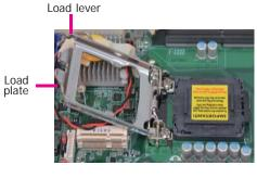
Remove the protective cap from the CPU socket. The cap is used to protect the CPU socket against dust and harmful particles. Remove the protective cap only when you are about to install the CPU.
