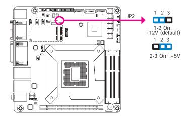
JP2 is used to select the power level of LVDS LCD inverter connector.
