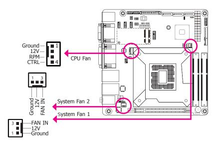
The fan connectors are used to connect cooling fans. The cooling fans will provide adequate airflow throughout the chassis to prevent overheating the CPU and system board components.
