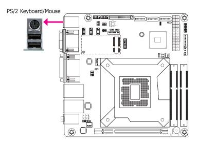
This rear I/O port is used to connect a PS/2 keyboard/mouse. The PS/2 mouse port uses IRQ12.
