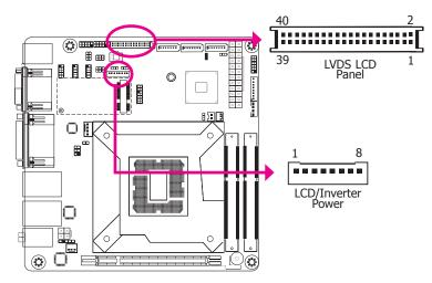
The system board allows you to connect a LCD Display Panel by means of the LVDS LCD panel connector and the LCD/Inverter power connector. These connectors transmit video signals and power from the system board to the LCD Display Panel.
