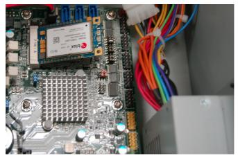
2. Push the Mini PCIe card down and use the provided mounting screws to secure the card on the system board.
