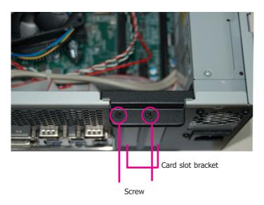
2. Insert the expansion card in the connector on the motherboard and press down until secured.
