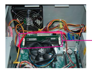
The installed DIMM
