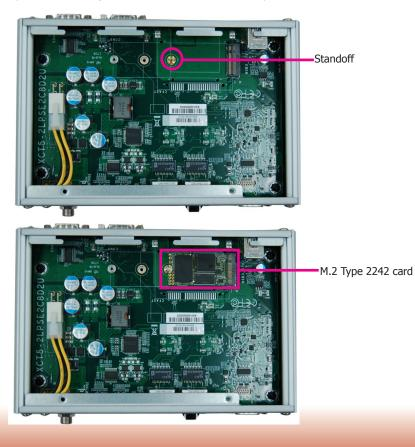
Chapter 3 Installing the Devices
