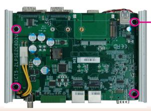
Remove these screws to detach the expansion board from the main board
