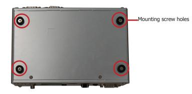
2. Use the provided mounting screws to attach the wall mount brackets to both sides on the bottom of the system.
