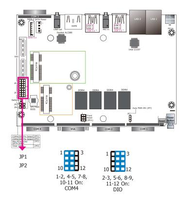
The system board uses JP1 and JP2 to select between RS232 serial communication or 8-bit DIO for the DB-9 connector (COM 4) at the rear panel.
