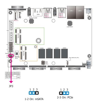
JP3 is used to select the signal for the half-size Mini PCIe slot: PCIe or mSATA (default).
