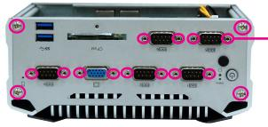
Use a wrench or a screwdriver with a socket end to remove the fasteners used on DB-9 and VGA connectors.
