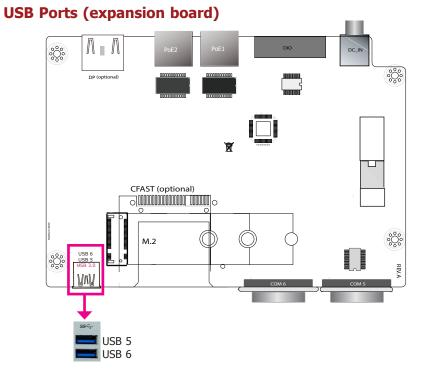
The expansion board is equipped with two onboard USB 3.0 ports (USB 5-6). USB devices allow data exchange between your computer and a wide range of simultaneously accessible external Plug and Play peripherals.
