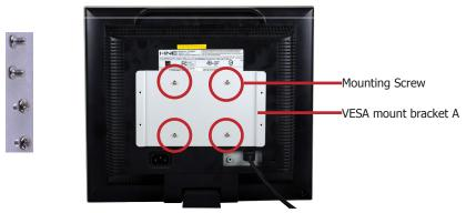
3. Align VESA bracket A with VESA bracket B, and then use the provided mounting screws to attach both brackets to secure the system in place.
