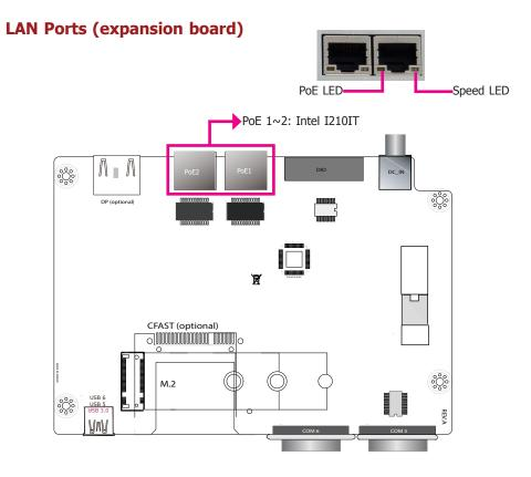
PoE LAN 1 and LAN 2 are PoE (Power over Ethernet) ports and are built on the Intel® I210IT PCI Express Gigabit Ethernet controller. With PoE (Power over Ethernet) support, the ports carry power to connected devices without the need for individual power supplies. Each port delivers up to 15.4 Watts of power to the connected devices that comply with IEEE 802.3af, for example, access points and VoIP phones.
