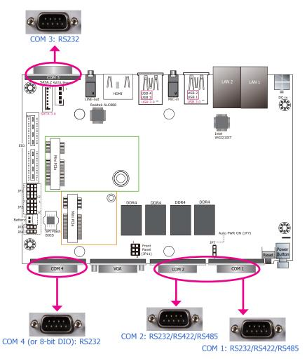
COM 1 and COM 2 can be selected among RS232, RS422 and RS485 whereas COM 3 and COM 4 are fixed at RS232. Use the BIOS configuration utility to select the communication mode for COM 1 and COM 2.
