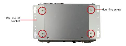
The following diagrams show the location and dimension of the wall moutning holes.
