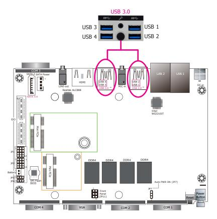
The system board is equipped with four onboard USB 3.0 ports (USB 1-4). USB devices allow data exchange between your computer and a wide range of simultaneously accessible external Plug and Play peripherals.
