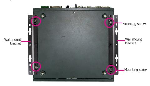
The following illustration shows the location and dimension of the holes for mounting the device onto a wall or rack .
