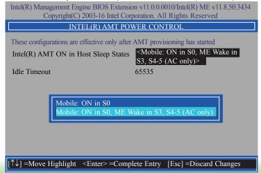
50. In the **Intel(R) AMT Power Control** menu, select **Idle Timeout** then press Enter. Enter the timeout value and press Enter.
