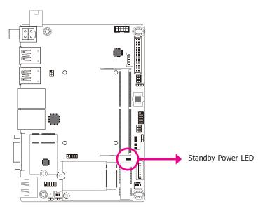
This LED will lit red when the system is in the standby mode. It indicates that there is power on the system board. Power-off the PC and then unplug the power cord prior to installing any devices. Failure to do so will cause severe damage to the motherboard and components.
