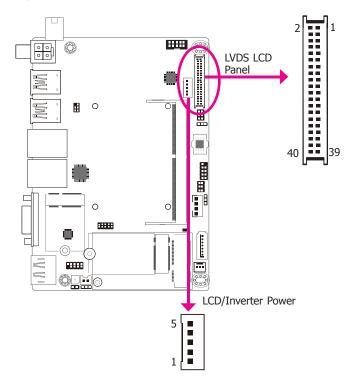
The system board allows you to connect a LCD Display Panel by means of the LVDS LCD panel connector and the LCD/Inverter power connector. These connectors transmit video signals and power from the system board to the LCD panel.
