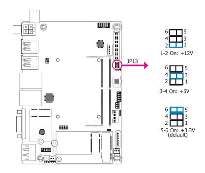
JP13 is used to select the power supplied with the LCD panel.
