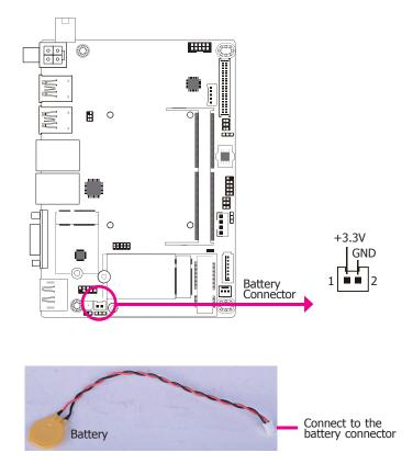
The lithium ion battery powers the real-time clock and CMOS memory. It is an auxiliary source of power when the main power is shut off.
