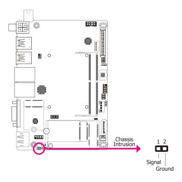
The board supports the chassis intrusion detection function. Connect the chassis intrusion sensor cable from the chassis to this connector. When the system's power is on and a chassis intrusion occurred, an alarm will sound. When the system's power is off and a chassis intrusion occurred, the alarm will sound only when the system restarts.
