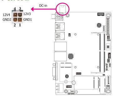
This 4-pin right angle connector is considered a low power solution. Connect a DC power cord to this connector. Using a voltage more than the recommended range may fail to boot the system or cause damage to the system board.
