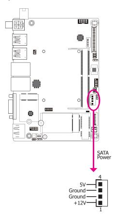
The SATA power connector supplies power to the SATA drive. Connect one end of the provided power cable to the SATA power connector and the other end to your storage device.
