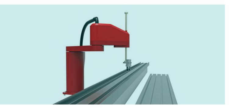
SCARA (Selective Compliance Assembly Robot Arm or Selective Compliance Articulated Robot Arm) is a specially configured robot arm. It is a new assembly robot concept proposed by a Japanese manufacturer in 1981. A small load characterizes it. On the other hand, the speed is fast, so it is mainly used in fast sorting, precision assembly, other 3C industry, the food industry, and other fields.
